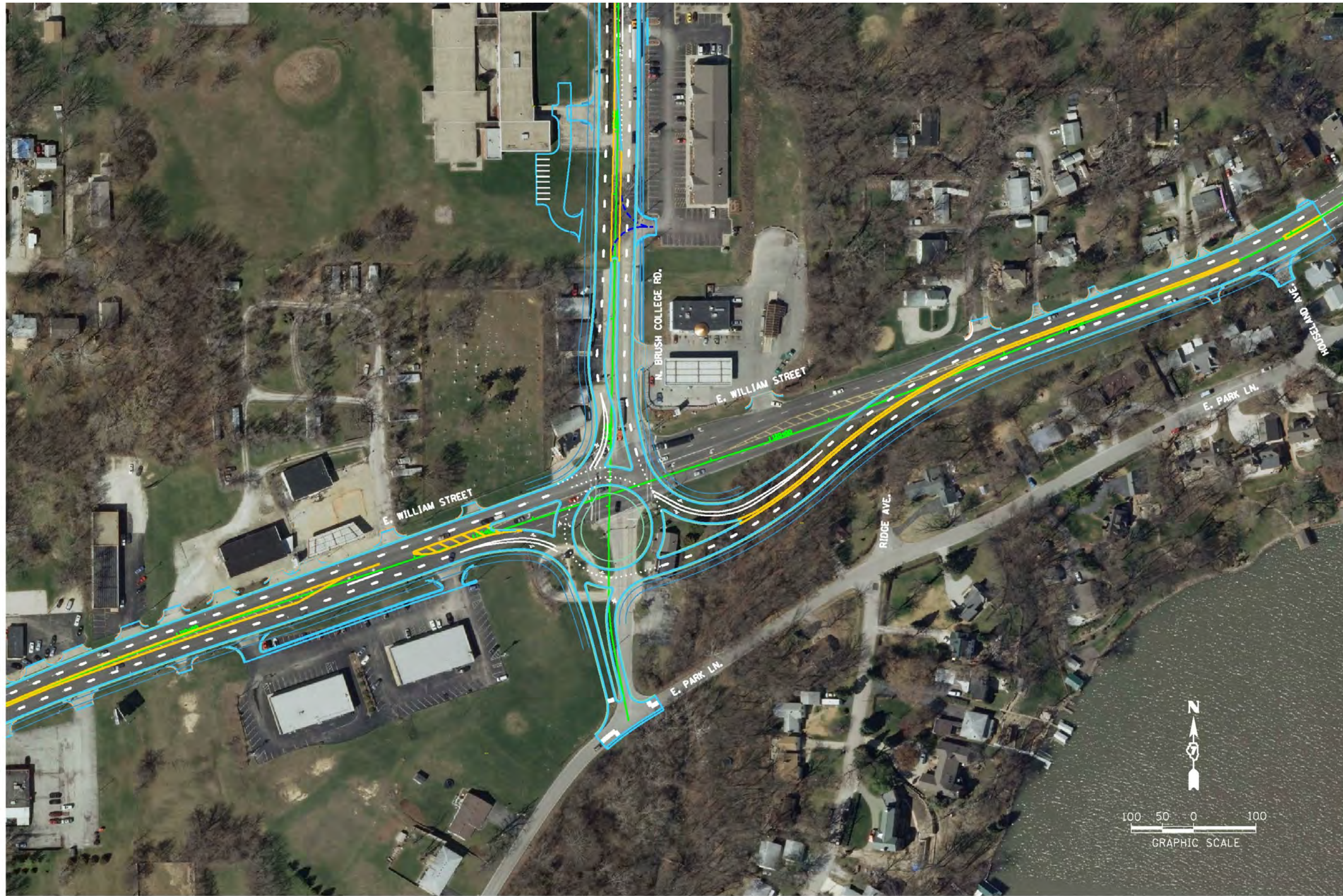
Figure 10 – Williams Street (IL 105) Intersection – Roundabout Option
