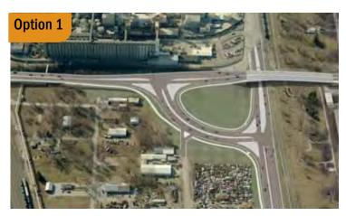
Option 1 consists of a ramp from Brush College Road to Faries Parkway, with traffic signals at the top and the bottom of the ramp. A free-flow right turn lane is provided from northbound Brush College Road to Faries Parkway.
